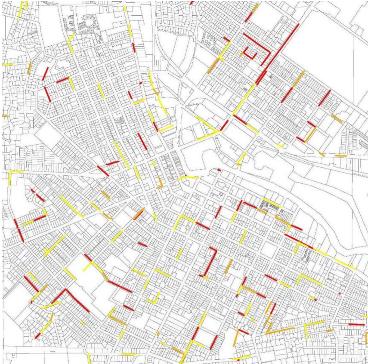
Figure 10: Sample of Sewer Main Conditions
