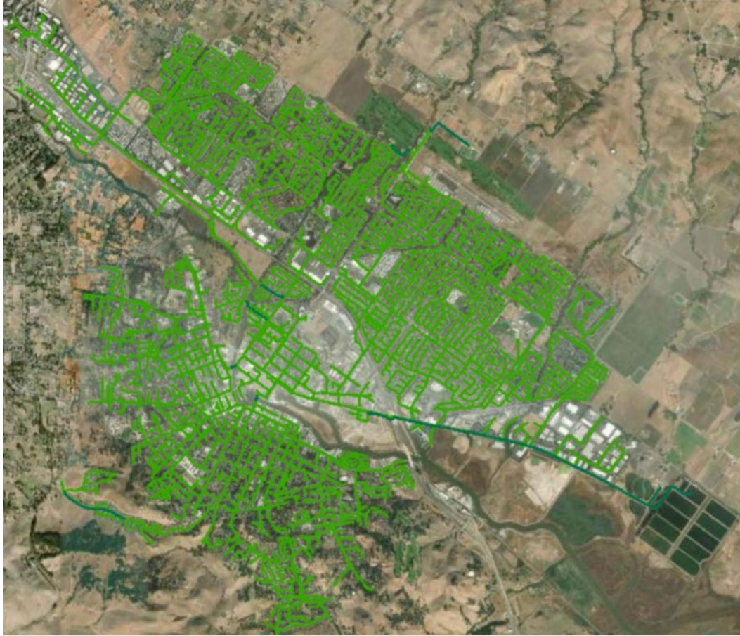
Figure 7: Sewer Mains within the City of Petaluma
